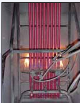
Bunched cables being tested for fire retardance .
