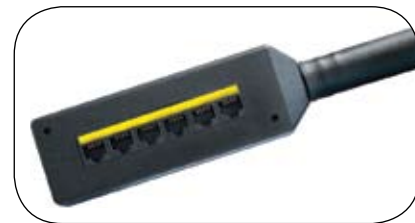
Ex: 25ZD/5E6BTS-100 = 25 Pair Cable Assembly, Zone Distribution module to Telco Straight, Cat 5e Riser, 568B wired, 100 Feet
