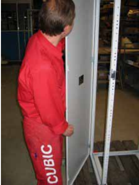
6. Sides and backpanel are all lifted on the hinges, closed and locked at the droplock brackets on the cornerprofiles.
