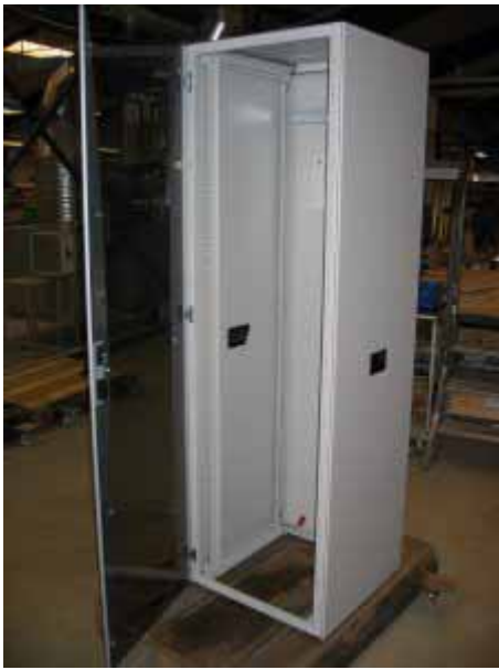
7. The door is mounted on hinges and closed.
